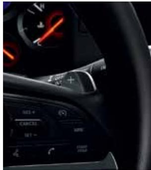
Two clutches. No clutch pedal. A lightening-quick shift. Inside Nissan GT-R's 6-speed dual-clutch transmission, the clutches work together. When the car's in an odd-numbered gear (1st, 3rd, 5th), the even-numbered gear (2nd, 4th, 6th) is "pre-selected" and ready to make the shift immediately. The transmission is so smart, it even "blips" the throttle on downshifts to match rpm. Your left leg may not get much exercise, but you'll have great fun shifting the GT-R.
