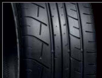
Even the design details of the GT-R's Dunlop SP Sport MAXX GT600 DSST CTT high-performance run-flat tyres are obsessive: a tiny block of rubber added to one of the treads combats tread squirm and gives a more confident, precise feel at the wheel.
